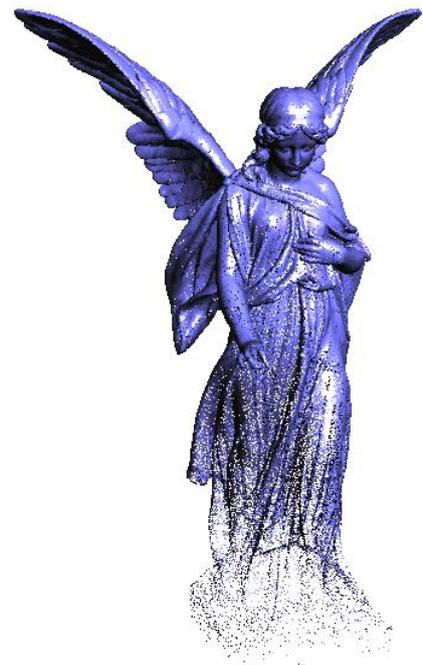
**Figure 1.** Example of the input set of points obtained by 3D scanning of a sculptural object and the final computer model. (the source: <http://www.cs.tau.ac.il/~dcor/>)
